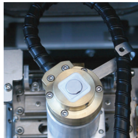
Standard Coolstage. Range: -30°C to +50°C at 300Pa
