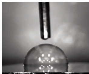
DDT modified Au surface before Glow Discharge. ca = 104.24°
