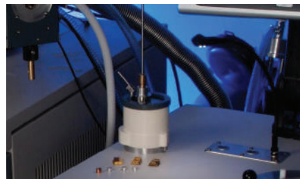
When not in use, the cryo transfer device can be stored under vacuum in the pumped storage tube, located on the Prepdek® work surface
