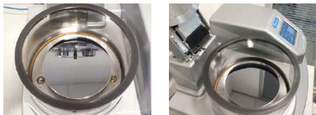
Q300T ES Plus has a 150 mm wafer capability
