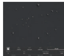
Molecular sieve particles applied from suspension onto carbon surface with Glow Discharge.
