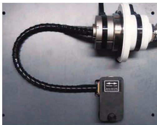
Coolstage and vacuum feed through connected to the storage block (stage protected by plastic shutter)
