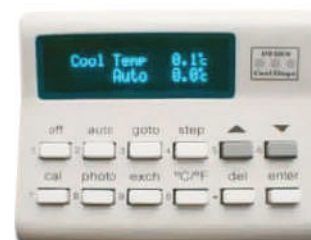
Ultra Coolstage. Range: -50°C to +50°C at 300Pa
