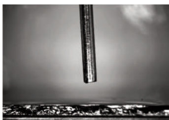
Carbon surface after Glow Discharge. ca = ~0°
