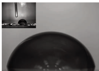
Carbon surface before Glow Discharge. ca = 66.55°
